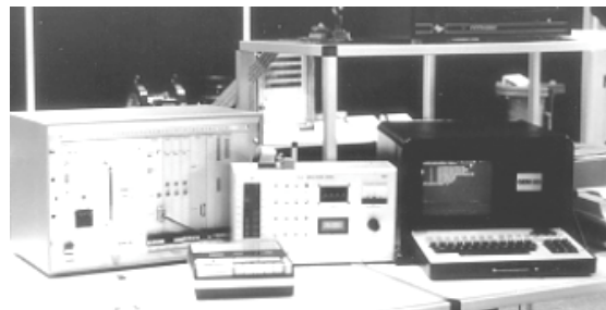
Early GEM80 kit - 200 series controller (with 8k RAM boards!), Simulation Panel and 8920 Portable Programmer. Programme data was stored on audio cassette prior to disks and PCs.
